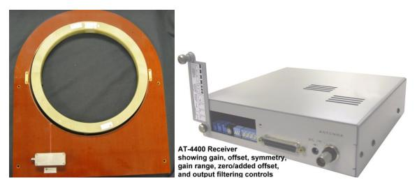
The picture on the left shows an AT-4400 split clamp-on collar for the 12.5" main drive shaft. For ruggedness, a phenolic stationary pickup coil was used (mahogany colored outer shape). A tuning enclosure can be seen on the lower left. A rear view of the Receiver is shown on the right. The Receiver's front panel has the on-the-fly shunt calibration switch.
